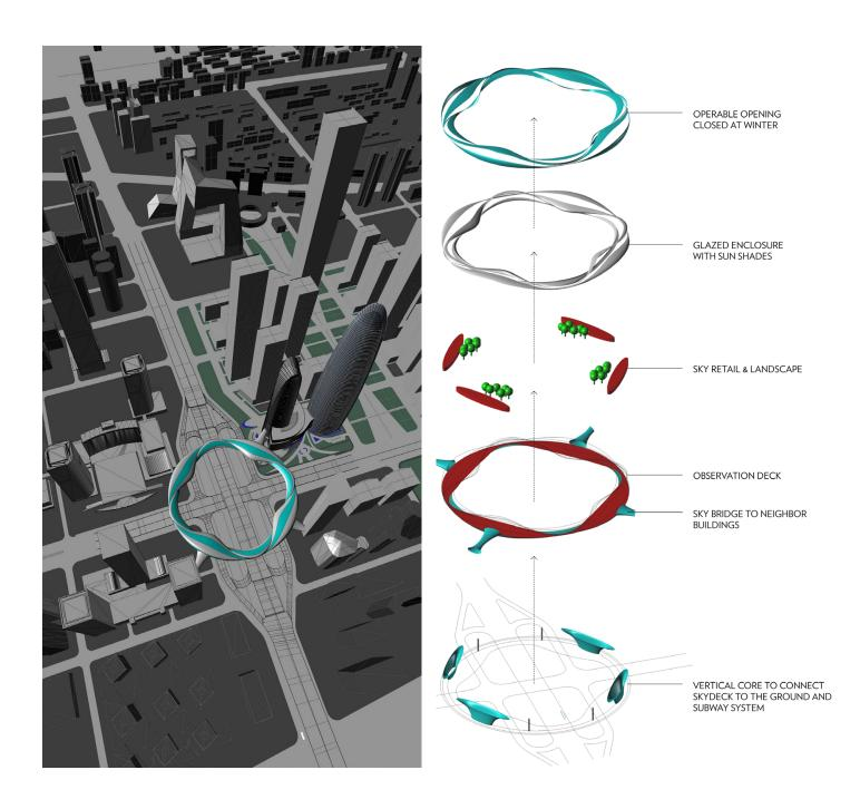
The proposed structural system for the Sky Ring is a composite structural steel braced system. The roof of the bridge will consist of a light structural steel system. The sky ring includes retail space around circulation cores (four thus) which also brace the structure of the bridge.
